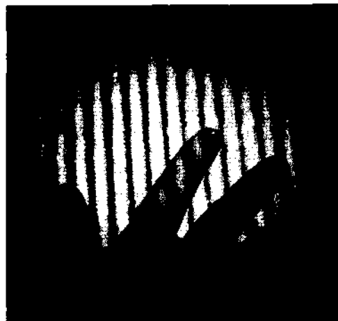
Real Michelson fringes using He-Ne laser light. (Photo by E. H.)
