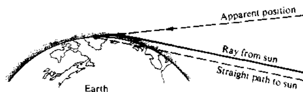
Figure 4.31 The bending of rays through inhomogeneous media. Because the rays bend as they pass through the atmosphere the Sun appears higher in the sky.
